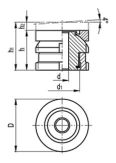
C-spanner DIN 1810 = A80-90 d = 39 D = 80 d1 = M60x2 For screw = M36 h = 94 h1 = 144
